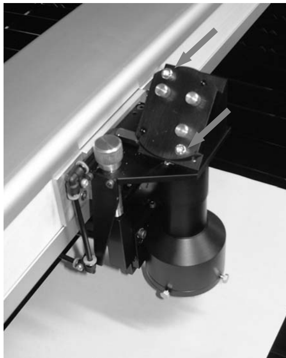
Figure 34: mirror #4 fixing screws
